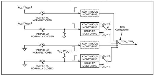
Figure 17: Tamper detect sampling options
