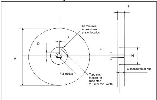
Table 25: Reel dimensions for 24 mm carrier tape (SOX28 package) and 16 mm carrier tape (SSOP20 package)
