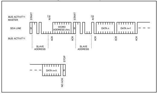
Figure 11: Alternate READ mode sequence
