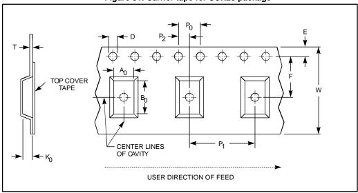
Table 24: Carrier tape dimensions for SOX28 package
