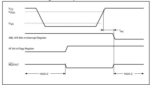
Figure 25: Backup mode alarm waveform
