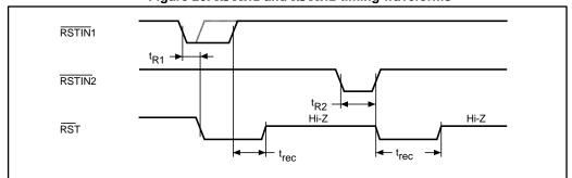
Figure 26: RSTIN1 and RSTIN2 timing waveforms
