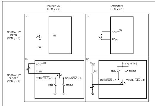
Figure 14: Tamper detect connection options
