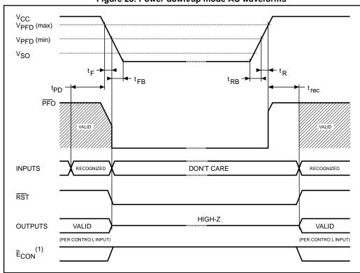
Figure 28: Power down/up mode AC waveforms
