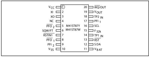
Note: No connect (NC) pin should be tied to V<sub>SS</sub>.
