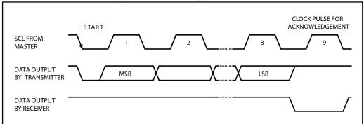
Figure 8: Bus timing requirements sequence
