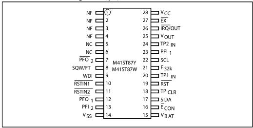
Note: No function (NF) and no connect (NC) pins should be tied to  $V_{\rm SS}$ . Pins 1, 2, 3, and 4 are internally shorted together.
