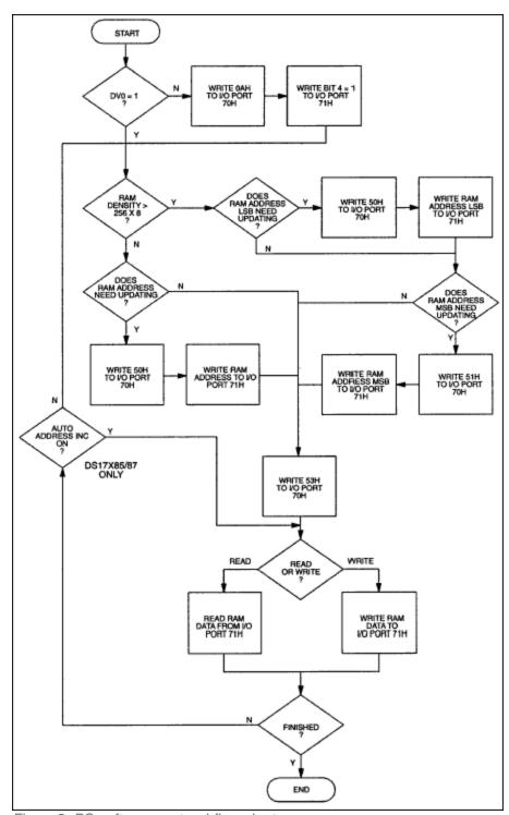
Figure 2. PC software protocol flow chart.
