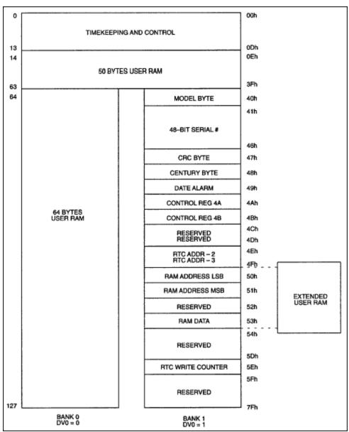
Figure 1. Register block partition.
