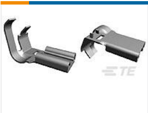
TE Part #42234-2 205 FASTON FLAG REC 20-14 AWG TPBR
