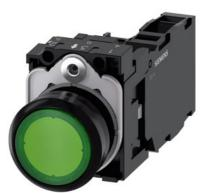
Illuminated pushbutton, 22 mm, round, plastic, green, pushbutton, flat, momentary contact type, with holder, 1 NO+1 NC, LED module with integrated LED 230 V AC, screw terminal, with laser labeling, inscription or symbol Customer-specific selection with SIRIUS ACT configurator (CIN)
