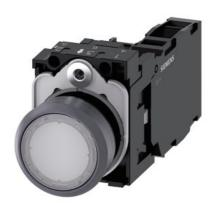
Illuminated pushbutton, 22 mm, round, plastic with metal front ring, white, pushbutton, flat, momentary contact type, with holder, 1 NO+1 NC, LED module with integrated LED 230 V AC, screw terminal, with laser labeling, upper case and lower case, always upper case at beginning of line
