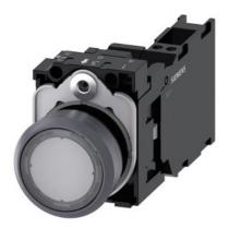
Illuminated pushbutton, 22 mm, round, plastic with metal front ring, clear, pushbutton, flat, momentary contact type, with holder, 1 NO+1 NC, LED module with integrated LED 24 V AC/DC, spring-type terminal, with laser labeling, upper case and lower case, always upper case at beginning of line
