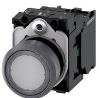
Illuminated pushbutton, 22 mm, round, plastic with metal front ring, clear, pushbutton, flat, momentary contact type, with holder, 1NO, LED module with integrated LED 24 V AC/DC, screw terminal, with laser labeling, inscription or symbol Customer-specific selection with SIRIUS ACT configurator (CIN)
