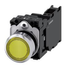
Illuminated pushbutton, 22 mm, round, metal, shiny, yellow, pushbutton, flat, momentary contact type, with holder, 1 NO+1 NC, LED module with integrated LED 110 V AC, spring-type terminal, with laser labeling, symbol number according to, ISO 7000 or IEC 60417
