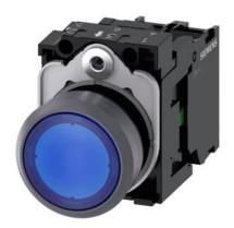
Illuminated pushbutton, 22 mm, round, plastic with metal front ring, blue, pushbutton, flat, momentary contact type, with holder, 1NO, LED module with integrated LED 110 V AC, screw terminal, with laser labeling, lower case
