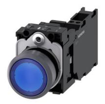
Illuminated pushbutton, 22 mm, round, plastic with metal front ring, blue, pushbutton, flat, momentary contact type, with holder, 1 NO+1 NC, LED module with integrated LED 24 V AC/DC, spring-type terminal, with laser labeling, inscription or symbol Customer-specific selection with SIRIUS ACT configurator (CIN)
