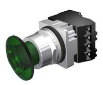
30mm Command/52, Chrome Finish Heavy Duty,Watertight/Oiltight Complete Metal Unit Illuminated Twist-to-Release Full Voltage, 120V AC/DC LED Lamp Mushroom Head Cap Small 1.79" (45 mm) Plastic Cap, Green 2 Position Maintained, Twist-to-Release with 1 N.O. - 1 N.C. Heavy Duty Contacts, A600/P600 UL Listed, CSA Certified NEMA 1,3,3R,4,4X,12,13 & Automotive Standards
