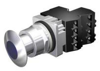
30mm Command/52, Chrome Finish Heavy Duty,Watertight/Oiltight Complete Metal Unit Illuminated Push-Pull Operator Full Voltage, 6V AC LED Lamp Mushroom Head Cap Small 1 3/4" (44.5 mm) Metal, Chrome with Blue Lens 3 Position Pull-Momentary/Push-Maintained 1 N.C.+1 N.C. Extra Late Break Heavy Duty Contacts, A600/P600 UL Listed, CSA Certified NEMA 1,3,3R,4,4X,12,13 & Automotive Standards
