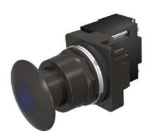
30mm BlackMax, Epoxy Coated Corrosion Resistant Complete Metal Unit Illuminated Push-Pull Operator Full Voltage, 120V AC/DC LED Lamp Mushroom Head Cap Small 1 3/4" (44.5 mm) Metal, Black with Blue Lens 3 Position Momentary UL Listed, CSA Certified NEMA 1,3,3R,4,4X,12,13 & Automotive Standards
