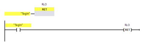
When the "TagIn" operand delivers signal state "1", the "Return" instruction is executed. Program execution is terminated in the called block and continues in the calling block.
