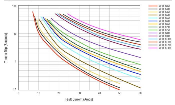
The Time to Trip curves represent typical performance of a device in a simulated application environment.
