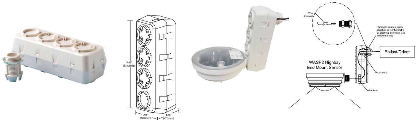
The Optional WSPADAPTOR2 offset adaptor can be used to improve the field of view for fixture mounted sensors where the geometry of the fixture might otherwise interfere with the sensor's performance. The adapter snaps into a standard 1/2" (12.7mm) knockout on the end of the fixture and provides several mounting position choices for the sensor.
