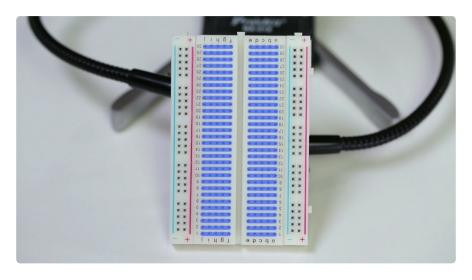
When we place a component on a breadboard, we're essentially wiring it into one of those internally connected rows.
