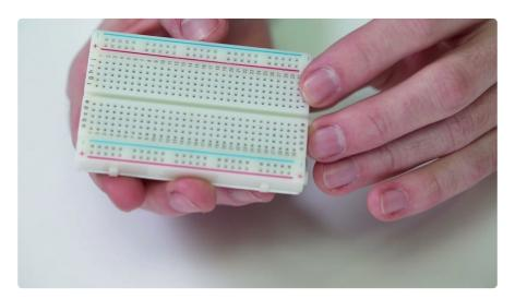
And in reality, a circuit usually exists on some type of circuit board - like say, a breadboard for example.
