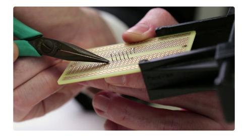
After placing a component on the board, bend its leads outward to keep it in place while soldering.
