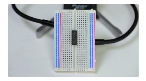
The two columns of holes along the sides are connected vertically.
