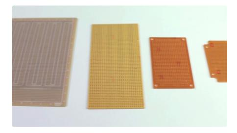
There are many different types available, but at the most basic level, perfboard is a perforated board - providing a grid of holes usually surrounded by metal "pads" which you can securely solder components to.
