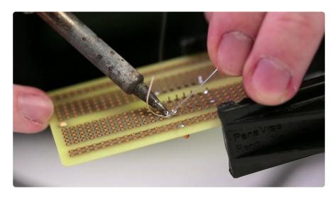
Because perfboard gives us access to the bottom side of our circuit, we can use the long component leads themselves to make some of the connections which required jumpers before.
