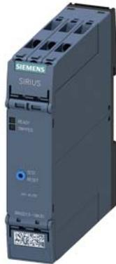
Thermistor motor protection relay Standard evaluation unit 22.5 mm enclosure screw terminal 2 change-over contacts US = 24 V AC/DC Manual/Auto/Remote reset with ATEX approval 2 LEDs (READY/TRIPPED) Safe galvanic isolation Test/reset button Wire break monitoring Short circuit monitoring non-volatile
