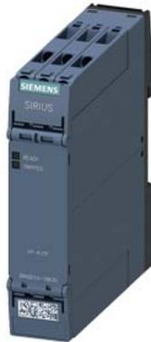
Thermistor motor protection relay Standard evaluation unit 22.5 mm enclosure screw terminal 2 change-over contacts US = 24 V AC/DC Auto-reset suitable for bimetallic switch 2 LEDs (READY/TRIPPED) galvanic isolation
