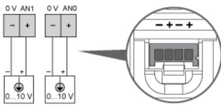
The (-) poles are connected internally.
