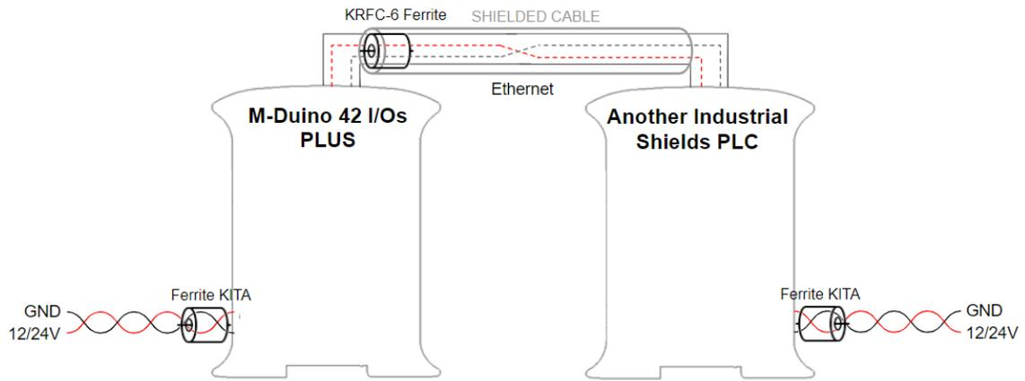
For an Ethernet communication between Industrial Shields equipment a **SFTP CAT-6 Ethernet crossover cable** must be used.
