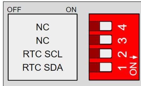
1. RTC SDA: This switch enables the communication to communicate with the RTC using I2C. Having this switch in ON mode it activates this communication, whereas if it is in OFF mode it disables the I2C to reach the RTC.
