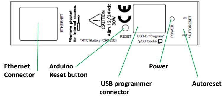
*\*NOTE: Autoreset. Arduino mega has auto reset when using serial communication code. Set switch to OFF when using serial communication. When uploading code to Arduino Mega set switch to ON.*
