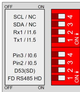
4. SCL/NC: **Always at OFF Position!** Switch has to be OFF position to enable SCL, **never ON** because in this position is NC (Not Connected).
