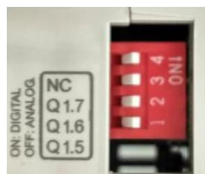
For the Analog Shield if a switch is set to ON, it can only act as Digital Output. If it is set to OFF it can only act as an Analog Output.
