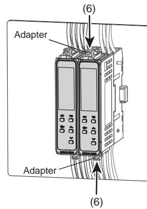
**Removing from the Mounting Panel**
