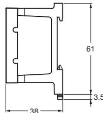
This Adapter is used to mount the E5CC-800 to a DIN Track. If you use the Adapter, there is no need for a plate to mount in the panel or to drill mounting holes in the panel.
