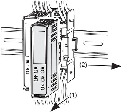
3. Remove the Terminal Units from the DIN Track.
