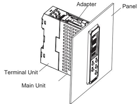
1. Insert the E5DC-800/E5DC-B-800 into the mounting hole in the panel. (Attach the Terminal Unit after you insert the Main Unit.)
