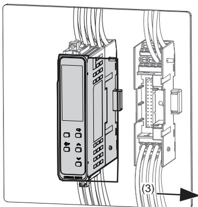
**Removing the Connector Cover
