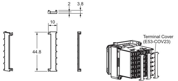
● Terminal Cover (for the P3GA-11 Back-connecting Socket)
