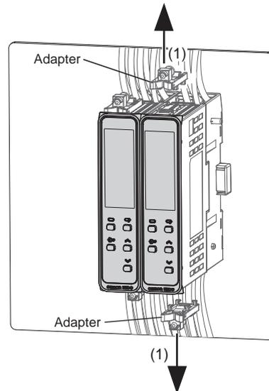
2. Remove the Main Unit from the Terminal Unit.
