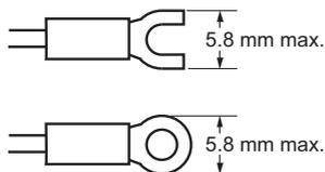
For the E5CC-U-800, use the following types of crimp terminals for M3.5 screws.
