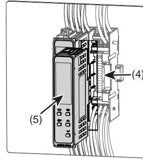
6. Push the adapter from the terminal unit side until it comes into contact with the panel to temporarily secure the unit, and then tighten the two fastening screws on the adapter. Alternately tighten the two screws little by little to maintain a balance. Tighten the screws to a torque of 0.29 to 0.39 N·m.
