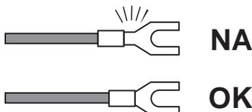
Although you can connect two crimp terminals with insulation sleeves to one terminal, you cannot do so if the diameter of the insulation sleeves is too large.
