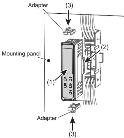
4. On the wired terminal unit, remove the connector cover on the side to use for connection to another terminal unit, and then connect the units together.
