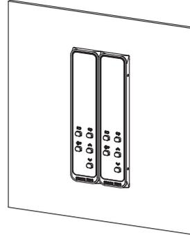
2. Peel off the release paper from the double-sided tape on the End Cover.
