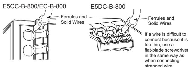
If a wire is difficult to connect because it is too thin, use a flat-blade screwdriver in the same way as when connecting stranded wire.
