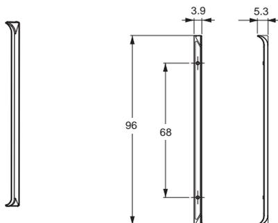
Use the End Cover when you mount the E5DC-800/ E5DC-B-800 to a panel to hide the gap between the Controller and the panel.
