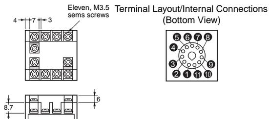
**Terminal Layout/Internal Connections (Bottom View)**
