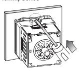
Mount the product on the panel, fasten bracket by pushing with tools as shown above.
