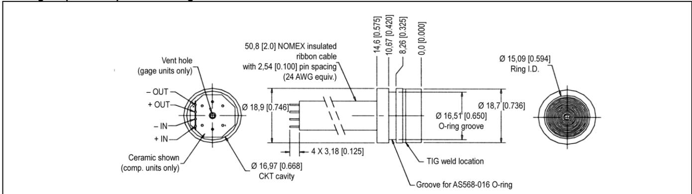
**Note:** Non-concentricity effects at the diaphragm weld area may cause runout of up to  $\pm 0.006$  in between the upper and lower portions of the sensor body. (It is recommended to use a counter bore to mate with this device to allow for this non-concentricity).
