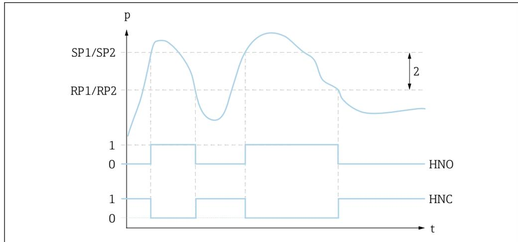
1 SP1/SP2: switch point 1/2; RP1/RP2: switch-back point 1/2
