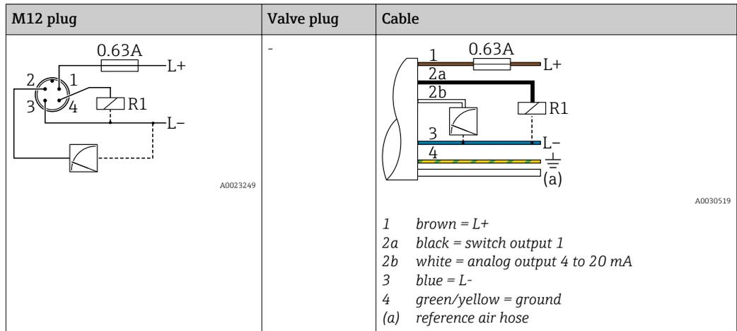
IO-Link: 1 x PNP switch output R1 with additional analog output 4 to 20 mA (active)
