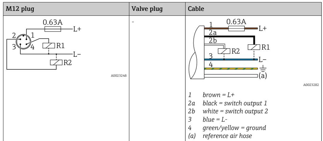
IO-Link: 2 x PNP switch output R1 and R2
