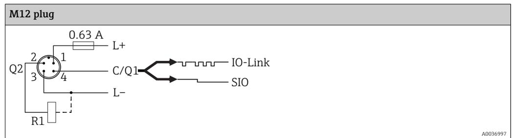
1 x PNP switch output R1 with additional analog output 4 to 20 mA (active)
