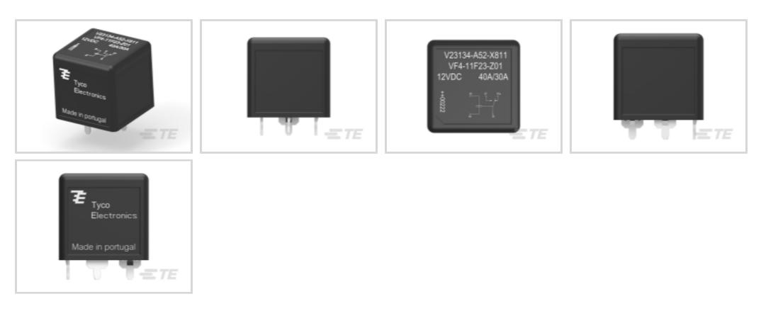
Coil Voltage Rating: 12 VDC Contact Current Class: **30 - 50 A** Contact Arrangement: 1 Form C (CO) Product Mount Type: Printed Circuit Board Coil Resistance: 90  $\Omega$
