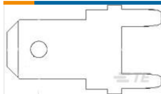
TE Part #1217057-1 187 FASTON,PCB TAB,TPBR
