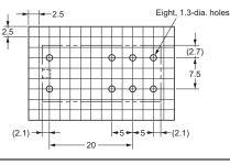
Terminal Arrangement/ Internal Connections (BOTTOM VIEW)
