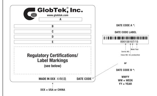
A=PoE, Passive Power Injector B=P/N: (料号) GT-96300-3648-T3-PP C=Model (型号) GT-96300-3648-T3-PP D=Input (输入)100-240V~, 50-60 Hz, 1.0A E=Output (输出)48.0 V == 0.75 A, 36.00W
