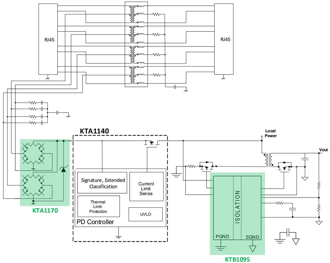
**Figure 5. KTA1140 High-Efficiency Synchronous Flyback DC-DC Solution with Isolated Controller**
