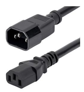
The PXT100143 C13 to C14 PDU Style Computer Power Extension Cord (3ft) features 14 AWG wire suitable for high power connections, making it a reliable solution for large server applications that require a higher rated, heavier gauge cable, and connecting to Power Distribution Units (PDU).
