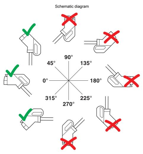
The resting position must be installed in the charging station such that the user cannot hang up the vehicle connector upside down (90° to 270°). However, positions rotated upward (45°) or downward (315°) are options for a resting position.
