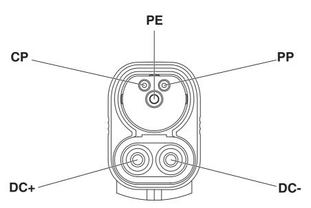
Pin assignment of the Vehicle Connector
