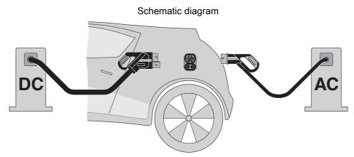
The Combined Charging System (CCS) principle - standard-compliant charging system for electric vehicles, which supports both conventional AC charging and fast DC charging. Both Vehicle Connectors fit into the CCS Vehicle Inlet.
