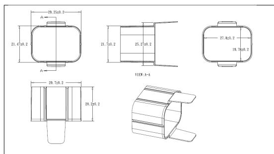
Warning: When removing connector with this sleeve included, take care not to damage the inlet when removing the connector. To remove the Sleeve that remains in the inlet after cord extraction, ensure the power cord is not plugged into power and use a non-conductive tool to extract.
