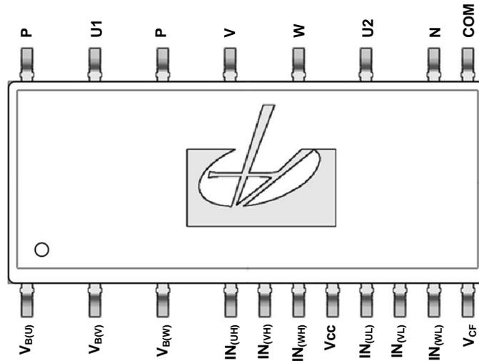
Figure 1. Pin Configuration
