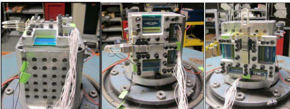
Figure 4 - Typical Mechanical Shock Test Setup
