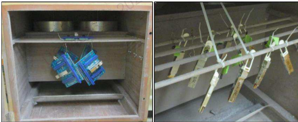
Figure 5 - Typical Benign Dust Contamination Test Setup
