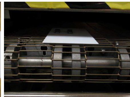
Figure 8 – Solderability Test Setup – Test Specimen on Oven Conveyor
