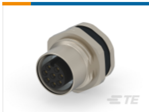
TE Part # T4171120008-001 M12,REAR MOUNT,FEMALE,A,8P,0.2 M WIRE
