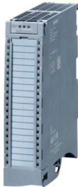
SIMATIC S7-1500 analog input module AI 8xU/I HF, up to 24 bit resolution, accuracy 0.1%, 8 channels in groups of 1; common mode voltage: 30 V AC/60 V DC, Diagnostics; Hardware interrupts Measured values scalable, measuring range adjustment, Calibrate in RUN; Delivery including infeed element, shield bracket and shield terminal: Front connector (screw terminals or push-in) to be ordered separately
