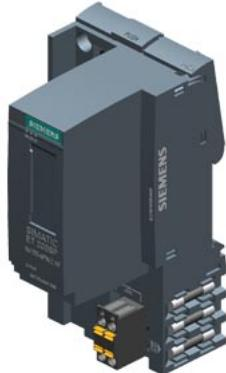
SIMATIC ET 200SP, PROFINET, 2-port interface module IM 155-6PN/2 High Feature, 1 slot for BusAdapter, max. 64 I/O modules and 16 ET 200AL modules, S2 redundancy, multi-hotswap, 0.25 ms, isochronous mode, optional PN strain relief, including server module
