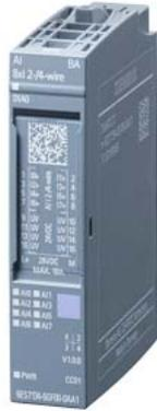
SIMATIC ET 200SP, Analog input module, AI 8xI 2-/4-wire Basic, suitable for BU type A0, A1, Color code CC01, Module diagnostics, 16 bit
