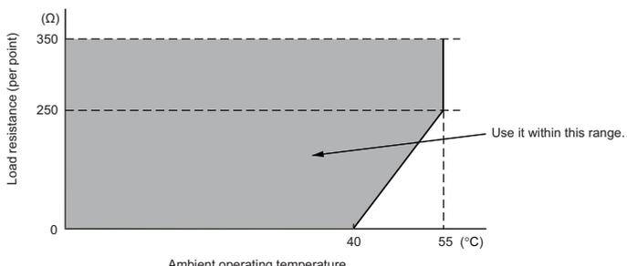
The graph shows the relationship between Load resistance (per point) and Ambient operating temperature. The y-axis represents Load resistance in Ohms (Ω), ranging from 0 to 350. The x-axis represents Ambient operating temperature in degrees Celsius (°C), ranging from 0 to 55. A shaded region indicates the allowed operating range, which is constant at 350 Ω up to 40 °C and then decreases linearly to 250 Ω at 55 °C. An arrow points to the shaded region with the text "Use it within this range."
