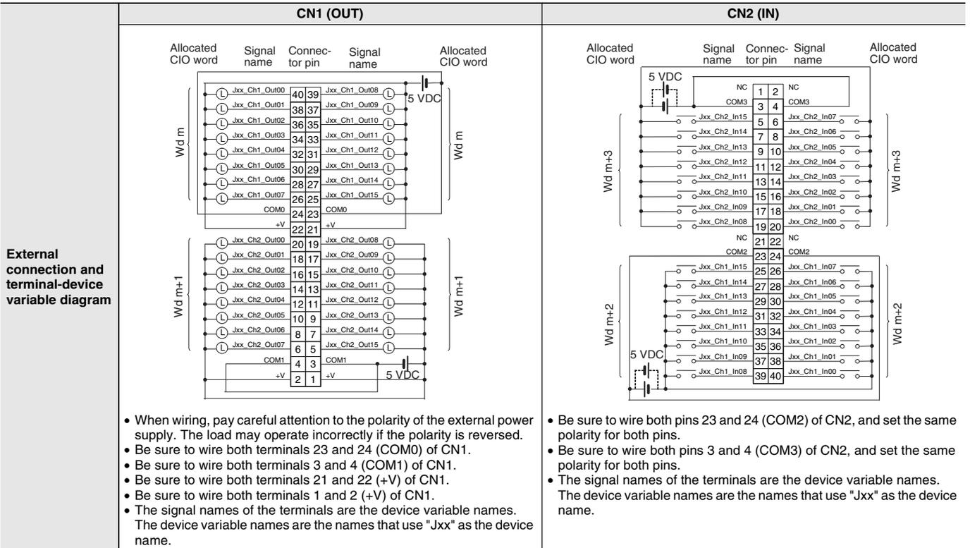
\* The ON response time will be 120 μs maximum and OFF response time will be 400 μs maximum even if the response times are set to 0 ms due to internal element delays.
