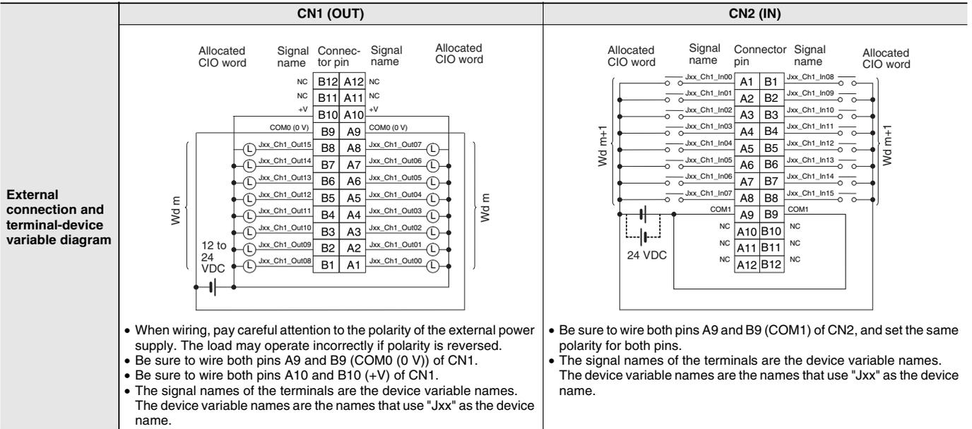
\* The ON response time will be 20 μs maximum and OFF response time will be 400 μs maximum even if the response times are set to 0 ms due to internal element delays.
