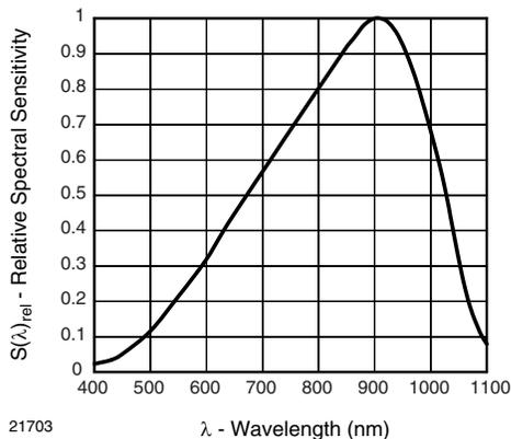
Fig. 1 - Relative Spectral Sensitivity vs. Wavelength
