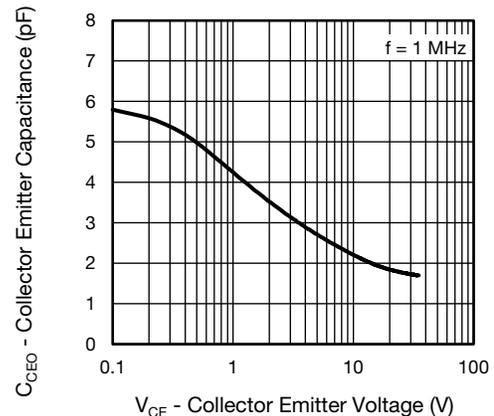
Fig. 2 - Collector Emitter Capacitance vs. Collector Emitter Voltage
