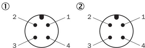
M12 male connector, 4-pin, A-coding
