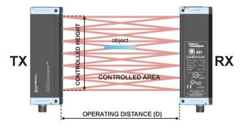
The beam interruption due to the passage of an object inside the controlled area causes the closing of the switching output and the variation of the device analogue output signal. Small objects can be detected (reaching dimensions of only 0.5 mm) and with a reduced surface area.
