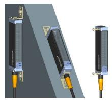
Mount the two receiver and emitter units on rigid supports which are not subject to strong vibrations, using specific fixing brackets and /or the holes present on the device lids
