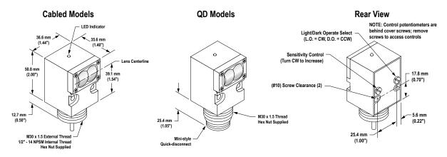
Note: Emitters have no light/dart operate switch, sensitivity control, or indicator LED.
