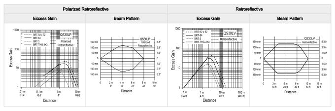
Fixed field performance is based on using a 90% reflectance white test card.
