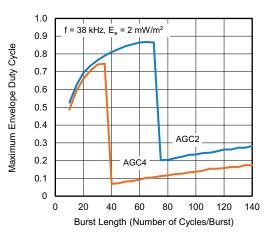
Fig. 8 - Maximum Envelope Duty Cycle vs. Burst Length
