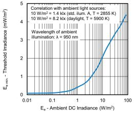
Fig. 6 - Sensitivity in Bright Ambient
