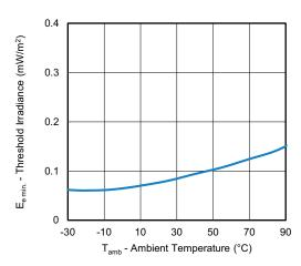
Fig. 9 - Sensitivity vs. Ambient Temperature
