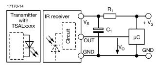
$R_1$  and  $C_1$  recommended in case there are strong ripple or spikes on the supply line.
