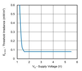
Fig. 12 - Sensitivity vs. Supply Voltage
