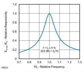
Fig. 5 - Frequency Dependence of Responsivity
