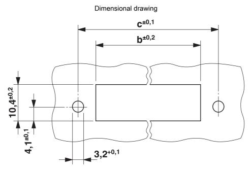
Dimension b: 10.49 mm + (no. of pos. x 5.08 mm) Dimension c: Dim. b + 9.27 mm
