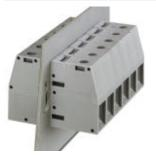
Panel feed-through terminal block, Connection method: Screw connection, Load current: 150 A, Cross section: 16 mm² - 50 mm², AWG 6 - 1/0, Width: 18.8 mm, Color: green-yellow
